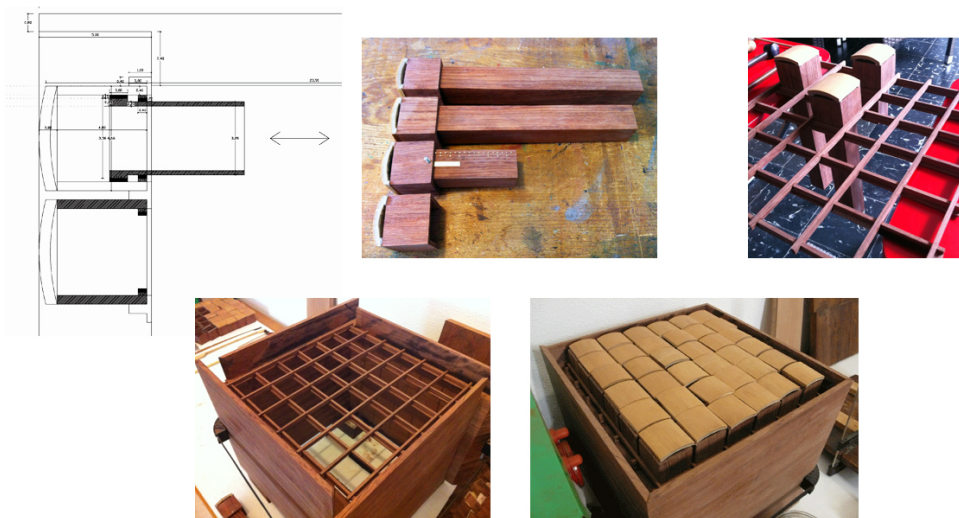
Fig. 4: Small echo chambers, retractable wooden tube and main acoustic box.
